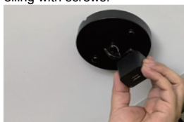
Step 4 Insert the transformer in the base.
